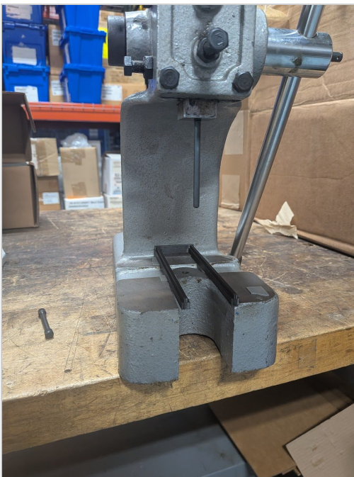
Fig. 4 — An arbor press set up with the fixture.
