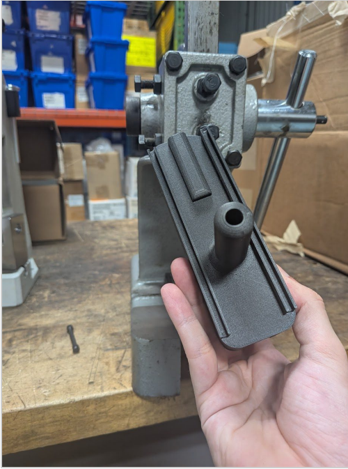
Fig. 6 — The 3D-printed fixture. The rail guides each part in and out.
