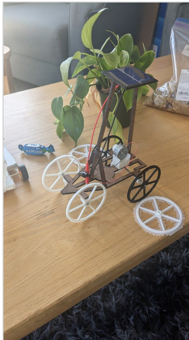
Fig. 1 — The finished solar rover. The panel sits on a mast above a light laser-cut frame.
