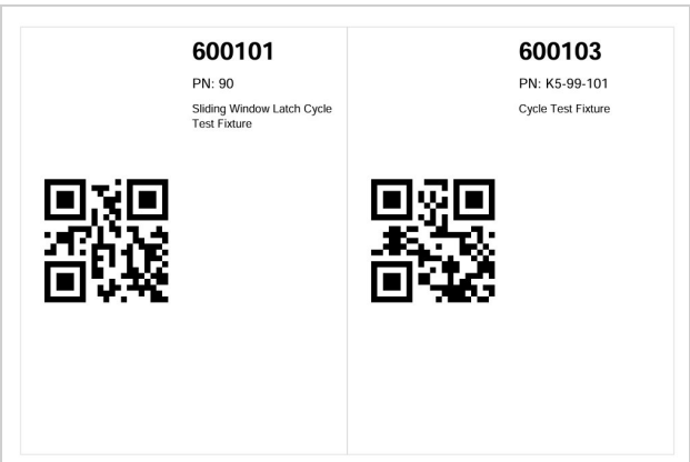
Fig. 3 —Printed labels. The QR encodes the serial number, so scanning it fills in the form.
