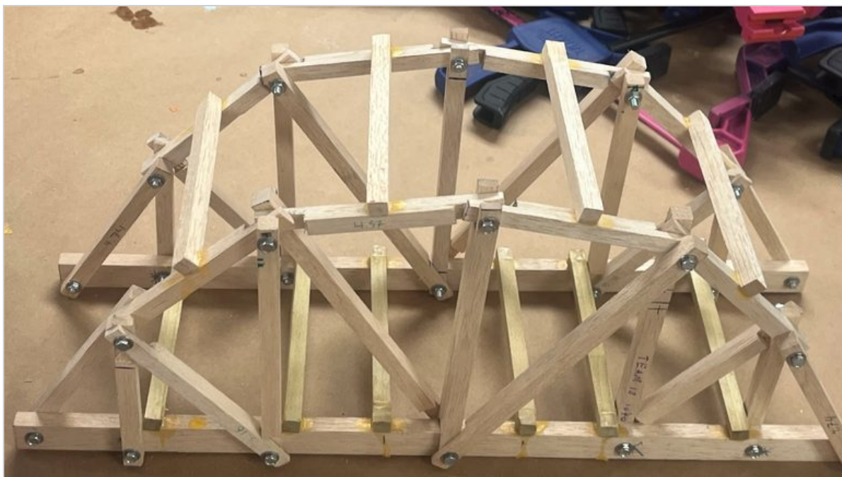
Fig. 1 — The built bridge. Balsa beams joined with bolts and washers, with the polygonal top chord of a Parker truss.
